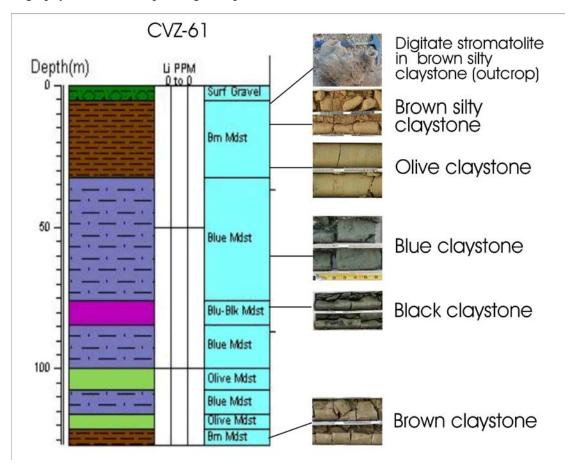
Figure 1. Stratigraphy and core photos for drill hole CVZ-61. This drill hole has 91 meters of lithium claystone in units of variable color. All of the claystone units except the brown silty claystone have relatively high lithium concentrations in previous drill holes on the property.
