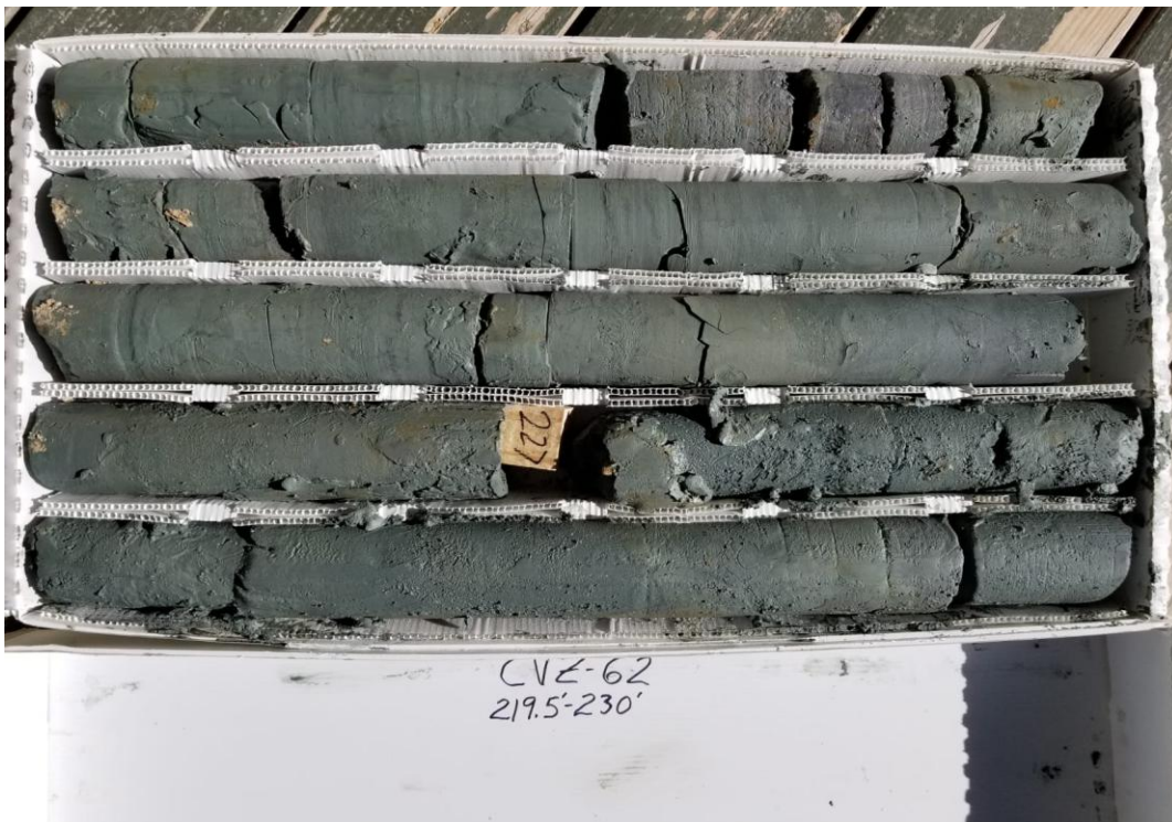
Figure 1 – core photos of blue claystone units from drill hole CVZ-62 between 219.5ft and 230ft (67m to 70m).
