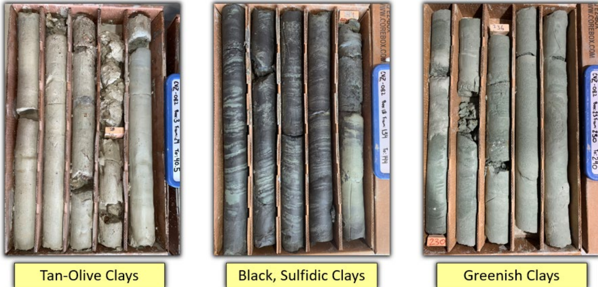
Figure 1 – CVZ-082 drill core examples of the various lithium bearing clay mineralization at Zeus.
